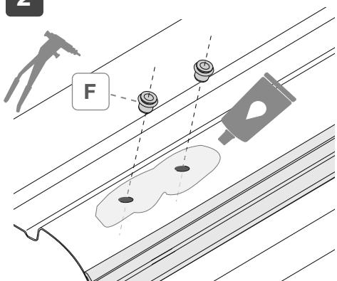
**EN** **Important:** use of SIKA 252 adhesive is essential for fixing the bracket (brackets).
